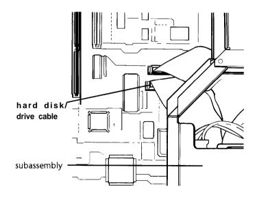
Grasp the connector and pull it straight up to remove it from the socket. Do not pull only on the cable.
